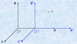
This fig. Shows two inertial frame of references one is stationary and other is moving with some constant velocity v.
